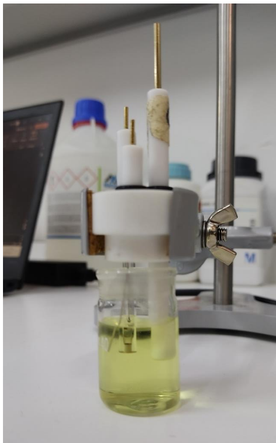
Figure 13: Three-electrode system with ferrocyanide
